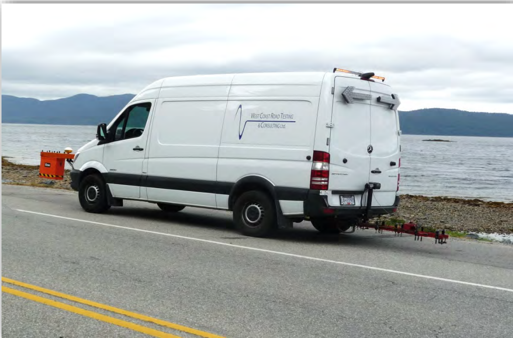
West Coast Road Testing FWD and GPR
